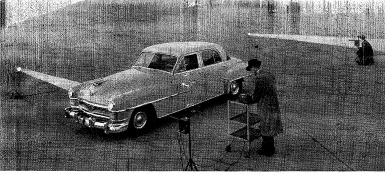
TIMED BY ELECTRIC EYE, Chrysler breaks light beams at start and finish of getaway test, while electronic machines measure
