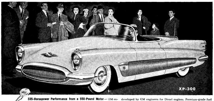
gineers developed an entirely new light alloy engine for these cars. It is a V-8, with 10 to 1 compression ratio, supercharged by a blower
